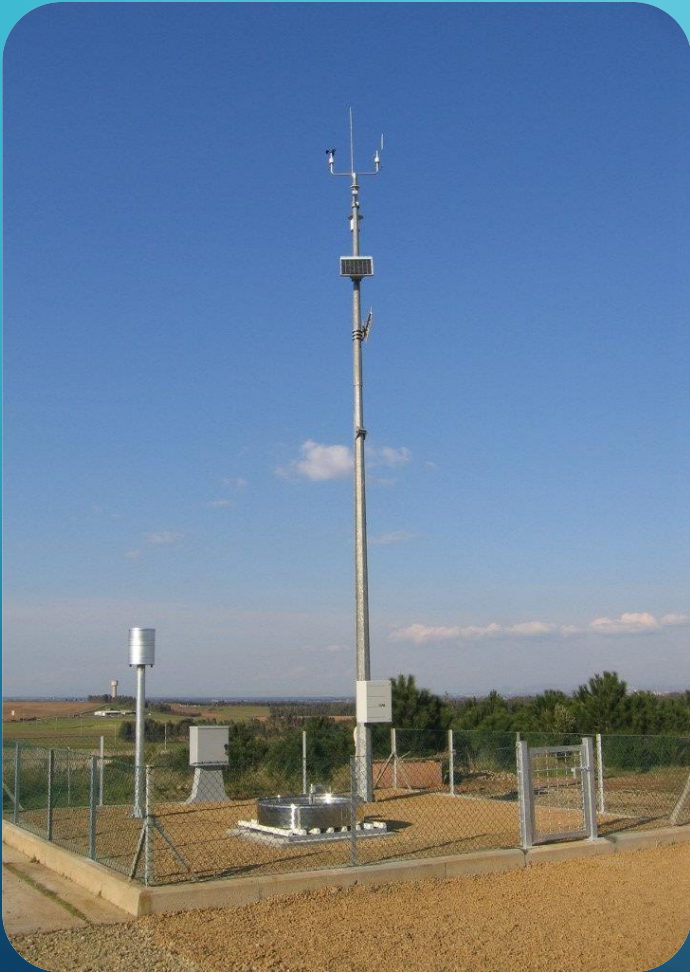
Standard solution 10m flippable mast
