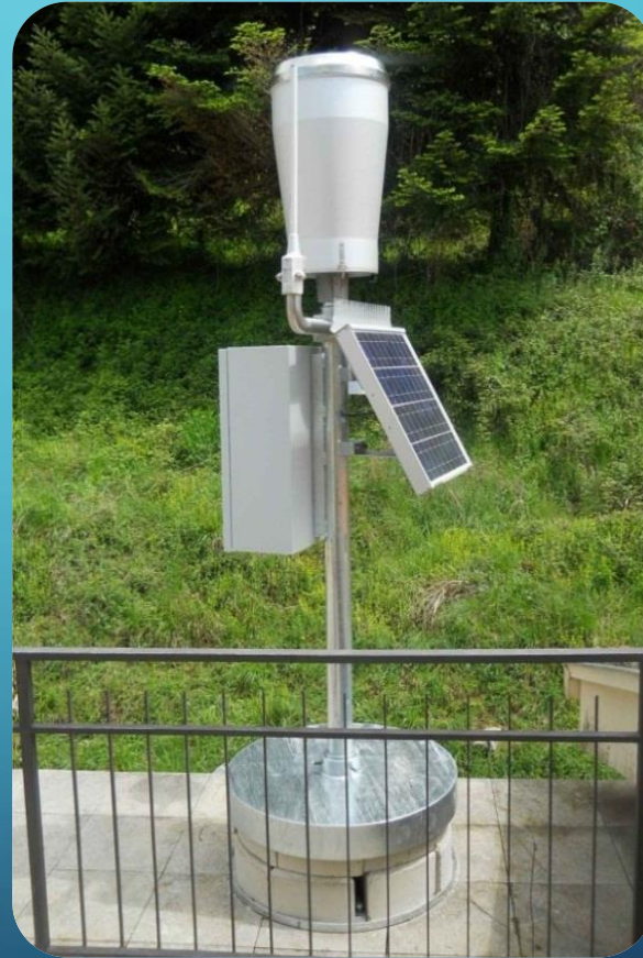
Portable solution Portable mast with dead weight
